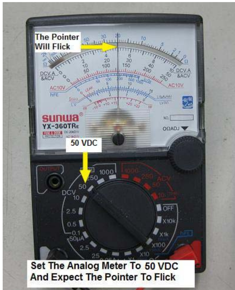
Figure 14.6- Expect The Pointer Of The Analogue Meter To Flick
