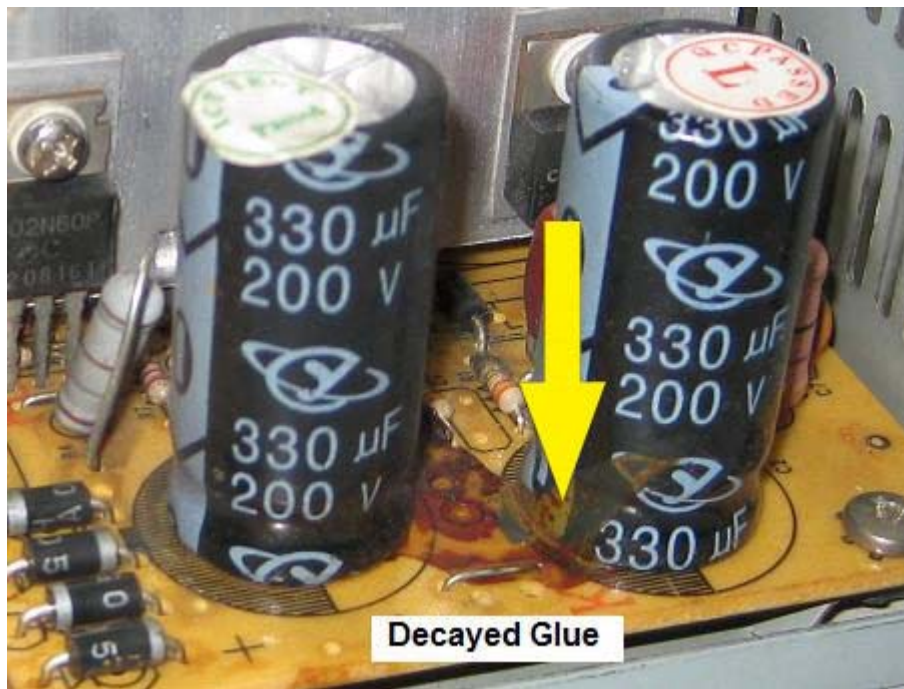
Figure 20.4- Decayed Glue Found In ATX Power Supplies
