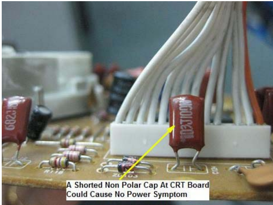
Figure 18.1- Shorted Non Polar Capacitor At CRT Board
