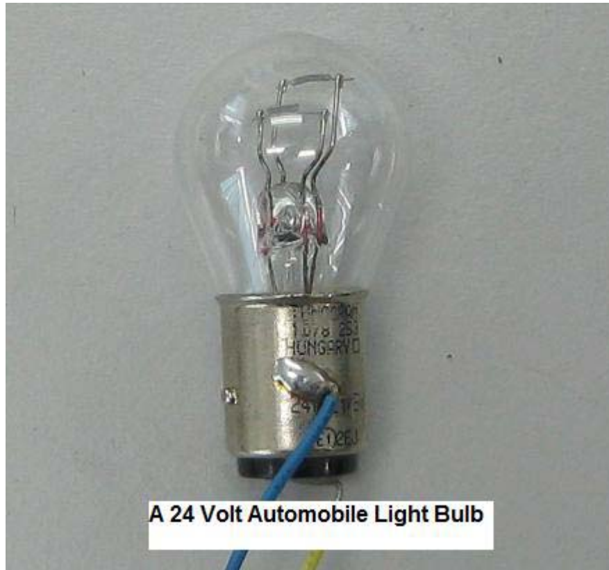
Figure 14.14- Use A 24 Volt Automobile Light Bulb As Load
