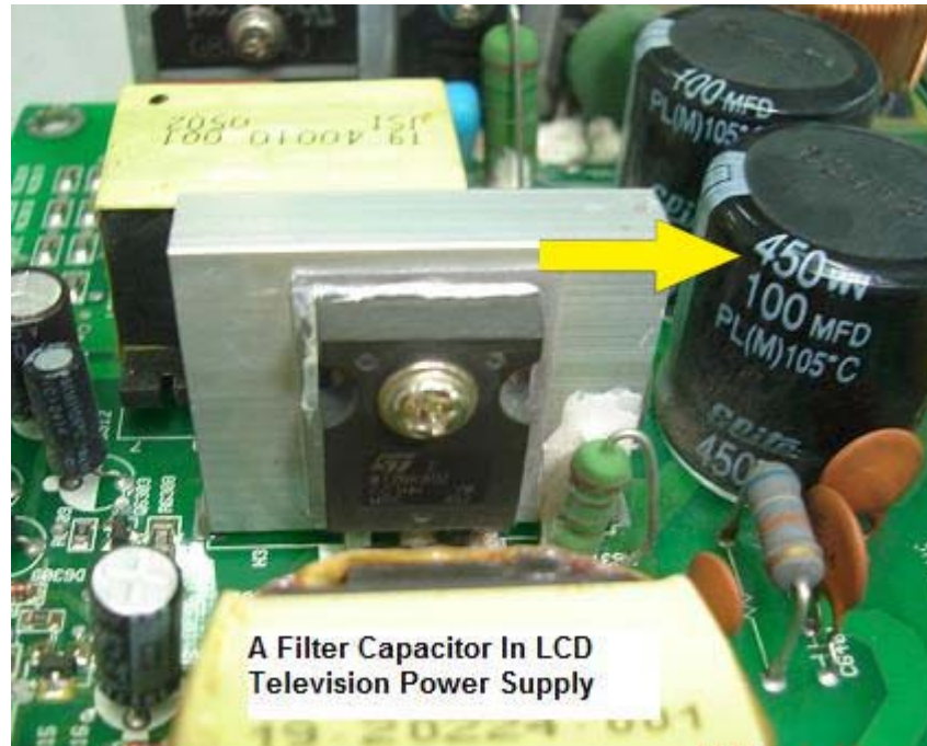
Figure 10.1- Filter Capacitors In LCD Television SMPS
