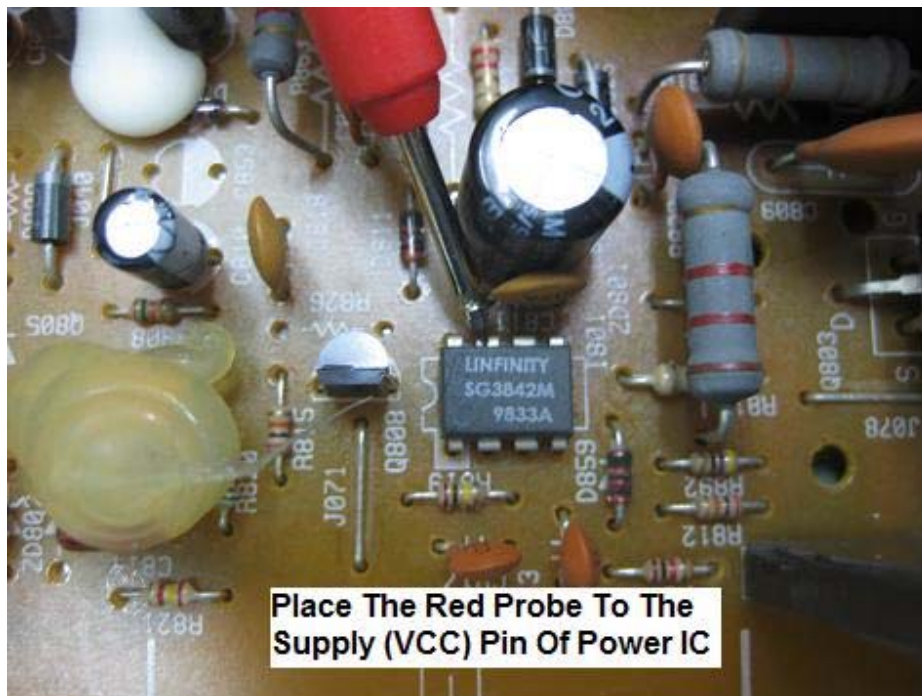
Figure 11.6- Testing Supply Voltage At The Power IC Pin
