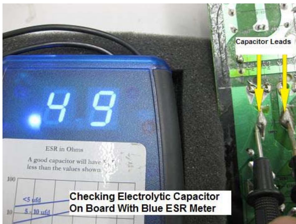
Figure 15.6- Blue ESR Meter Can Be Used To Test Filter Capacitors On Board
