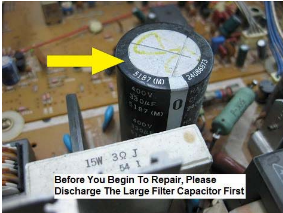
Figure 15.1- Discharge The Big Filter Capacitor With A 2.2 K Ohm 10 Watt Resistor Before You Start To Test On The Primary Side Components
