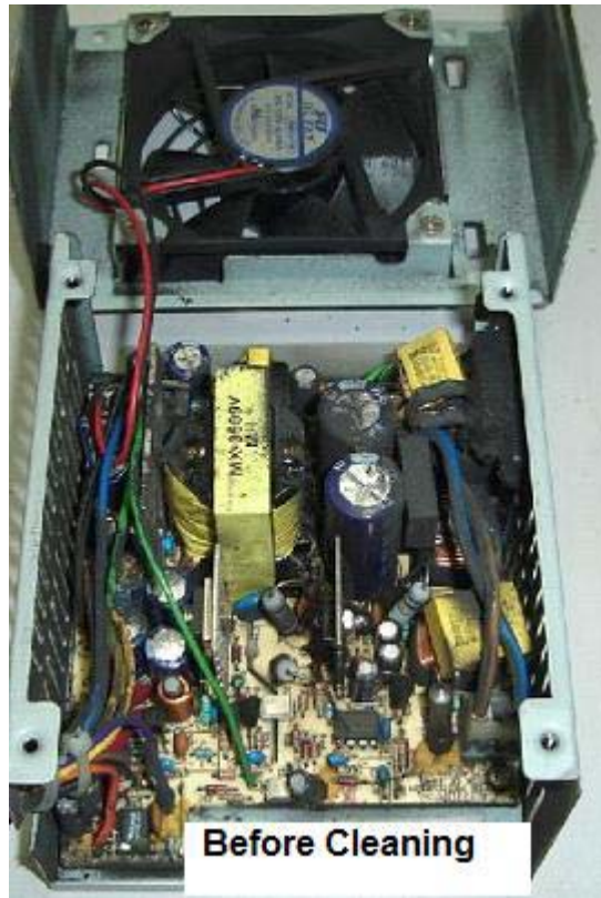
Figure 20.6- Dirt Inside The Power Supply
