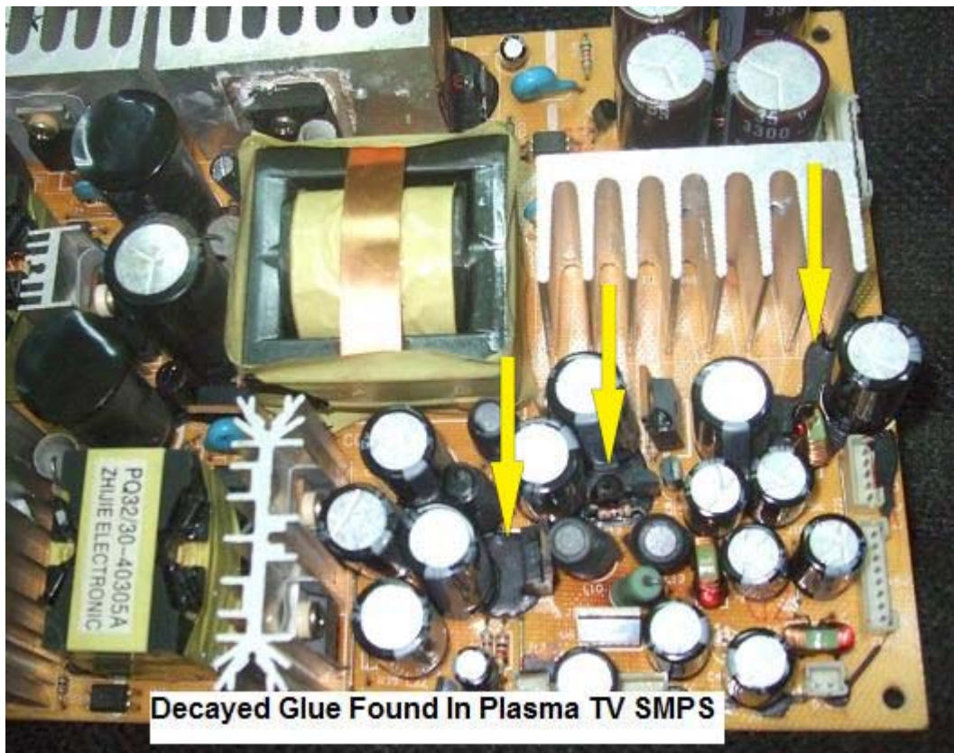
Figure 15.12- Decayed Glue Found In Circuit Board
